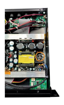
Be sure that the jumpers are applied to both left and right power supplies.
